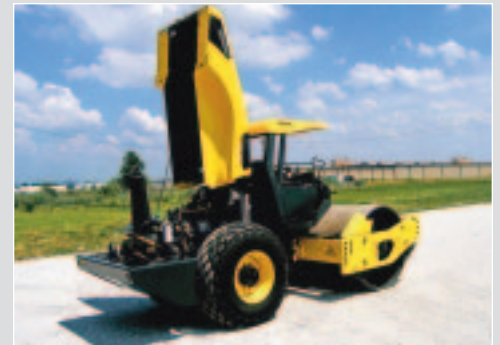
Vertically Opening Hood for Maximum Serviceability
